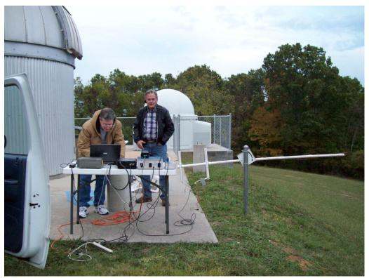
The following figure shows the equipment setup. From the left is the receiving down convertor (216.98 MHz to about 50 MHz), the power supply, the communications receiver tuned to about 50 MHz, and the laptop computer running a spectrum analyzer with a water fall display.
