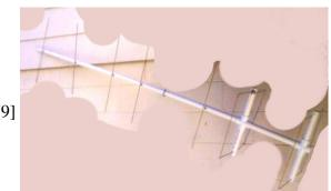
are used. Here's how it looked (on the left) in final 7-element form (last week, just in time for the Orionid meteor shower!
